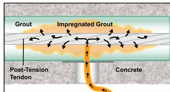
Fig. 2—Impregnation from a midpoint location on a tendon.
