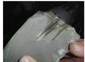
Fig. 15—Impregnation material present on outside surface of strands.
